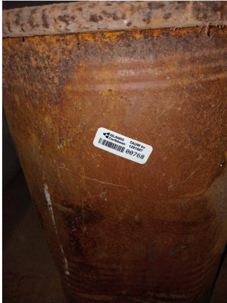
One of the zinc phosphide containers, carrying the inventory tag 00768, showing the advanced corrosion recorded in the factsheet.
