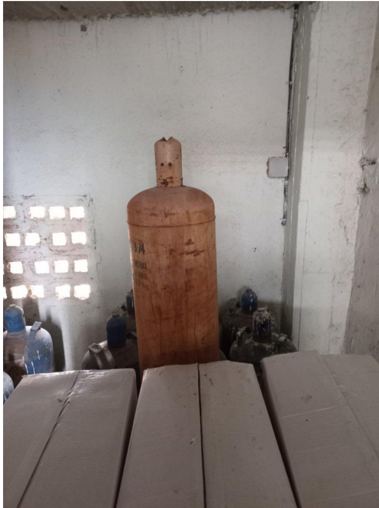
The empty methyl bromide cylinder, approximately 1.6 m tall and 50 kg (ref 00770).
